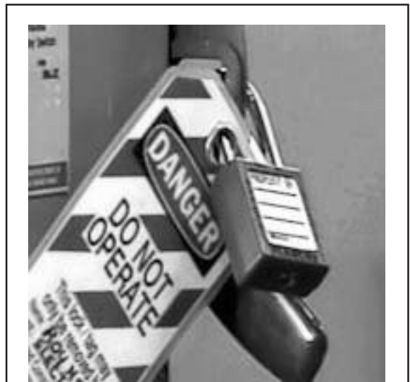
Figure 2: Equipment must be locked out and tagged out before preventive maintenance or servicing is performed.
